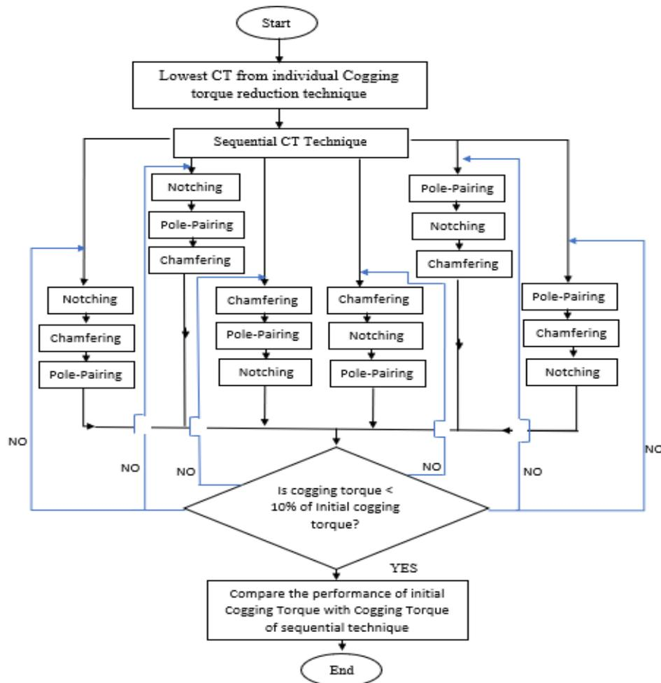
**Figure 6: Sequential cogging torque reduction technique process flow**
