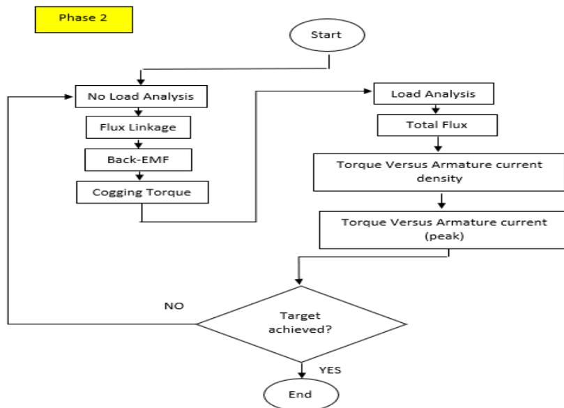
Figure 2: Flow of Performance Analysis of 4S-8P PMFSM
