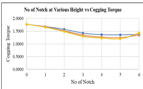
**Figure 10: Influence of the notch number on cogging torque of 4S-8P PMFSM topology**
