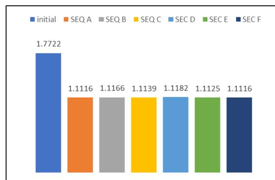
**Figure 14: The comparison of initial cogging torque with a cogging torque that undergoes sequential cogging torque reduction**
