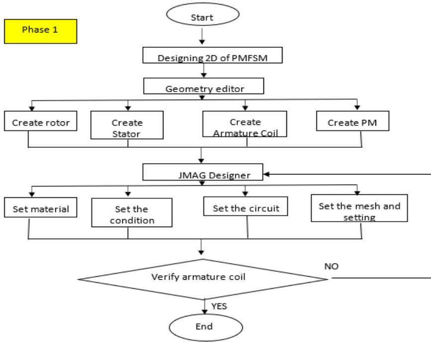
Figure 1: Process of Designing the 4S-8P of PM-FSM
