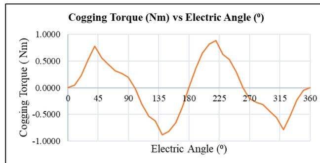
**Figure 8: Cogging Torque Analysis Performance**
