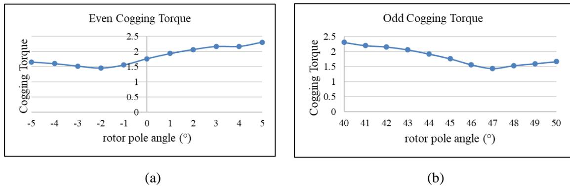
**Figure 13: The effect of even and odd pole against cogging torque**
