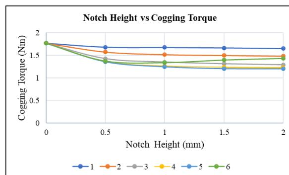
**Figure 11: Influence of the notch height on cogging torque of 4S-8P PMFSM topology**
