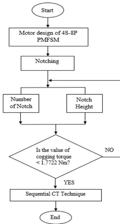
Figure 3: Process flow of notching technique
