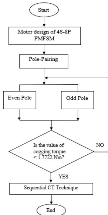
Figure 5: Process flow of pole pairing technique
