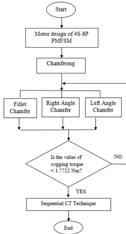
Figure 4: Process flow of chamfering technique
