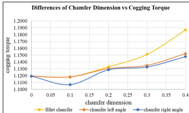
Figure 12: The cogging torque against different of chamfer dimensions
