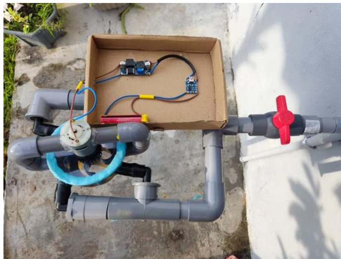
Figure 5: Top view of Pico hydro generator module
