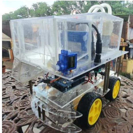
Figure 9: seeding part with complete assemble
