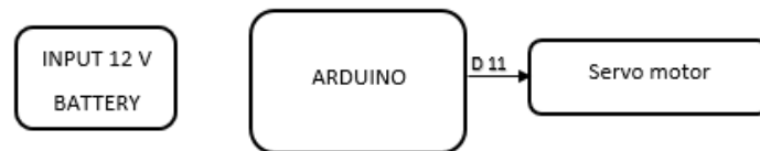
Figure 5: Connection for Servo Motor
