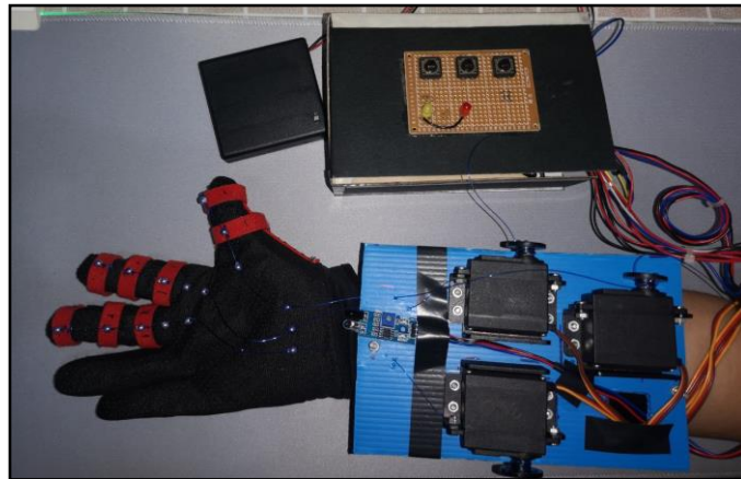
Figure 4: A fully assembled soft robotic hand glove to the microcontroller via wire.
