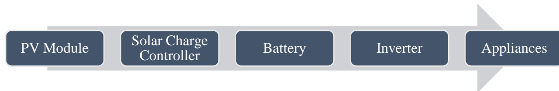
Figure 1: Process of OGPV system
