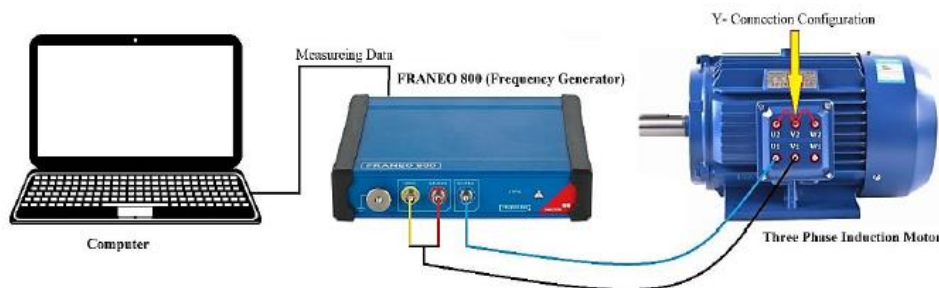
Figure 2: Equipment connection to measure response using FRA for motor winding [7]
