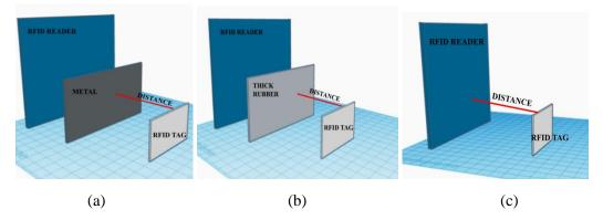
Figure 3: Hardware testing of RFID tagging system – (a) Metal as an obstacle (b) Thick rubber as obstacle and (c) Without obstacle
