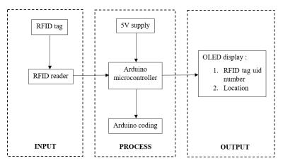
Figure 1: Block diagram of RFID tagging system
