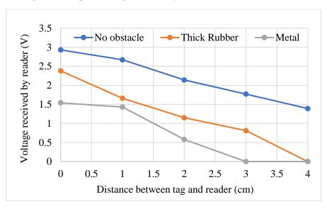
Figure 3: Graph of voltage received by reader vs distance (vertical)
