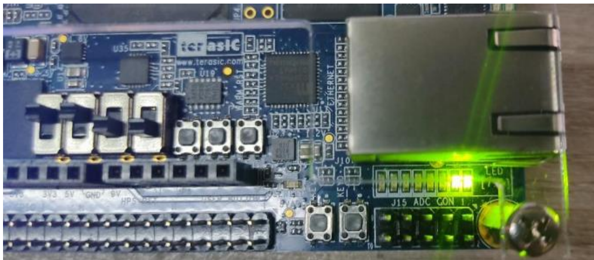
Figure 8: Switch is set to 100 and IN2= 1, IN1=1
