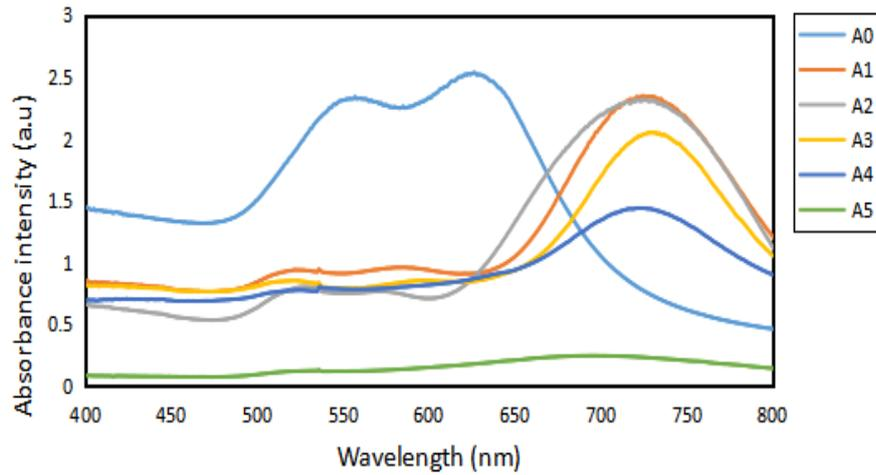
Figure 8: The optical response for various CTAB surfactant of GNRs
