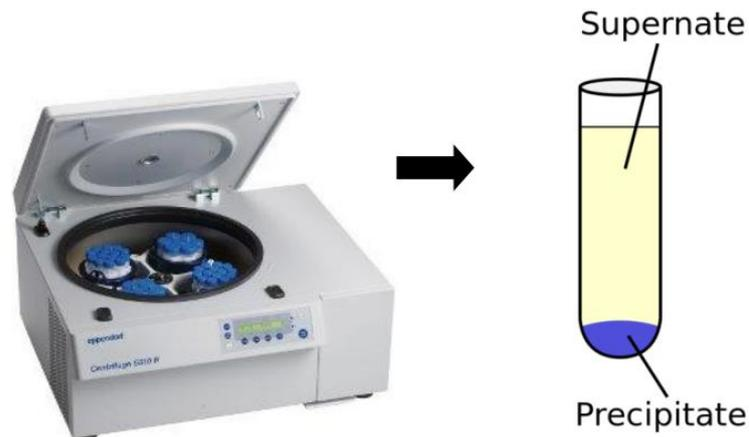
**Figure 2: Centrifugation process to separate the growth solution with a speed 5000rpm for 1 hour and a sample of separation precipitate and supernatant.**
