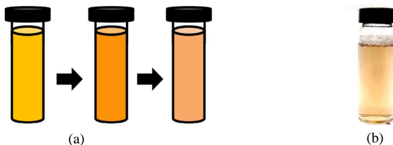
**Figure 4: (a) After mixed with three materials:  $\text{HAuCl}_4 \cdot 3\text{H}_2\text{O}$ , CTAB, and  $\text{NaBH}_4$  (b) After mixing the three ingredients, the seed solution changes colour to a light brown**
