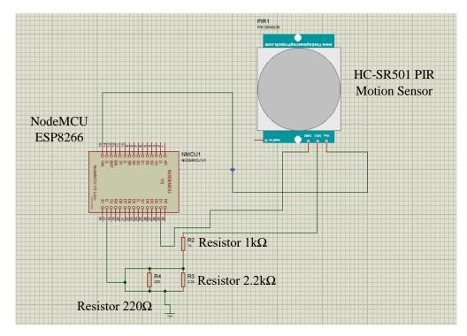
Figure 3: The Connection for IoT Based Child-in-Car Safety Reminder
