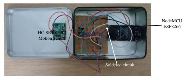
Figure 5: Circuit of the system that had been soldered
