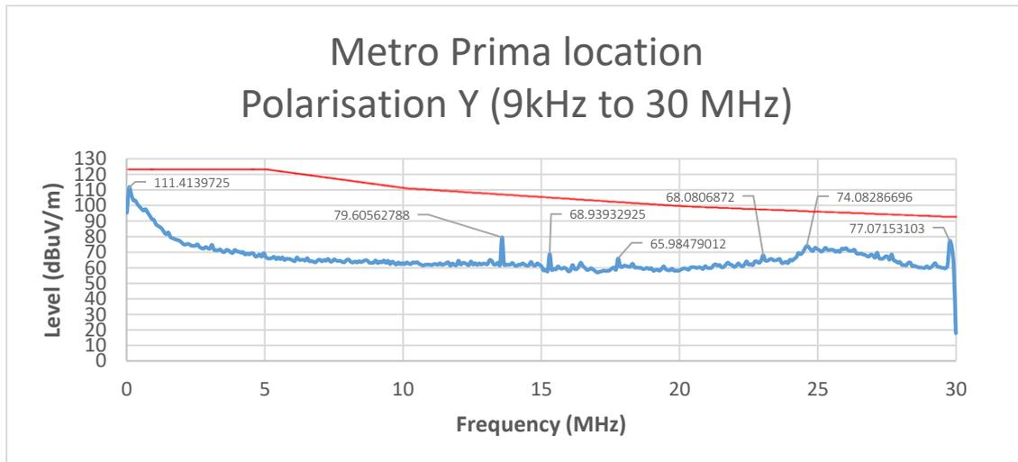
**Figure 8: Measurement result for polarization Y (9 kHz to 30 MHz)**
