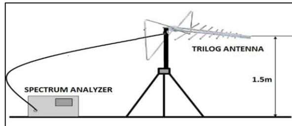
Figure 3: Test set-up for the tri-log antenna (30 MHz to 1 GHz)
