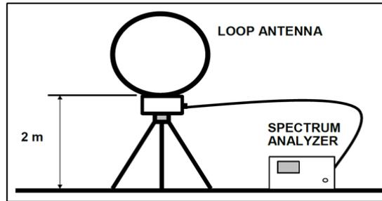
Figure 1: Test set-up for the loop antenna (9 kHz to 30 MHz)
