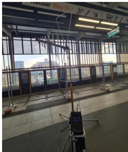
Figure 4: Real test set-up for the tri-log antenna at KVMRT 2 station
