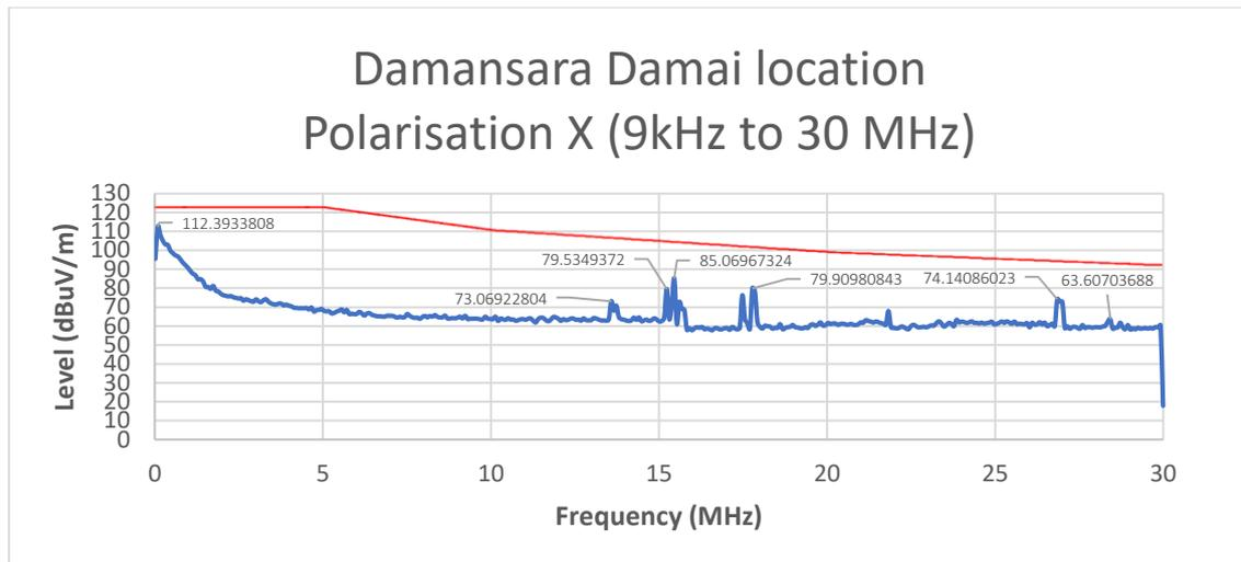
Figure 6: Measurement result for polarisation X (9 kHz to 30 MHz)
