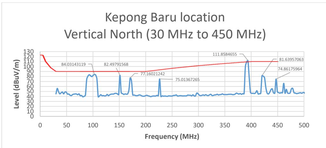
Figure 7: Measurement result for V-N (30 MHz to 450 MHz)
