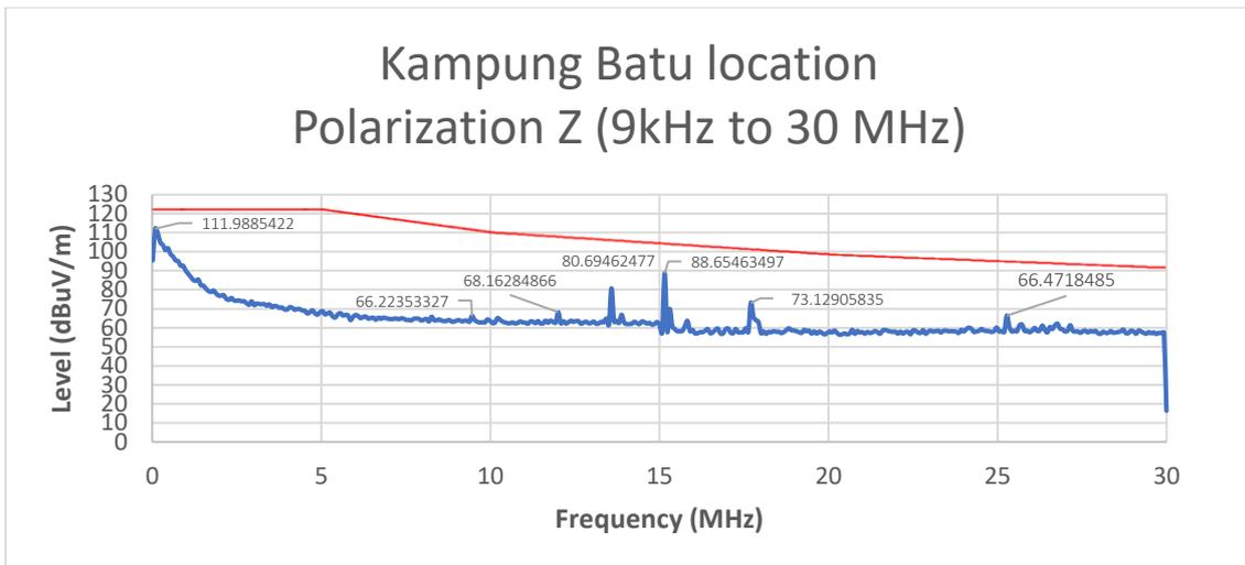
Figure 5: Measurement result for polarisation Z (9 kHz to 30 MHz)
