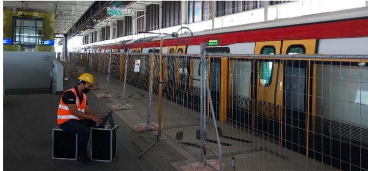
Figure 2: Real test set-up for the loop antenna at KVMRT 2 station
