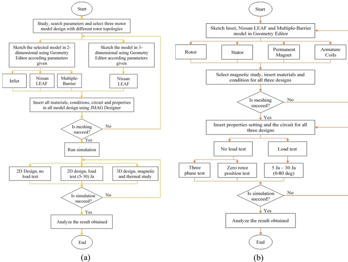
Figure 4: Flowchart of work for (a) general workflow of study (b) designing all 2-dimensional model
