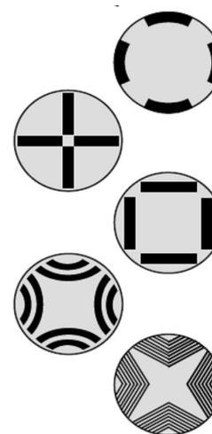
Figure 2: Different rotor type of IPMSM
