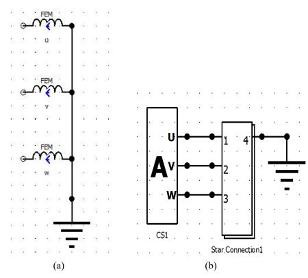
Figure 3: Circuit configuration for (a) no load test (b) load test
