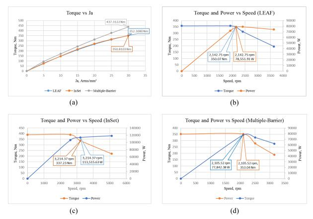
Figure 6: Result for load test of (a) toque vs Ja, (b)-(d) torque and power vs speed
