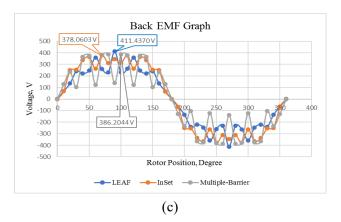
Figure 5: Result for no load test of (a) zero rotor position (b) cogging torque (c) back EMF
