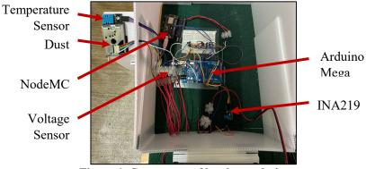
Figure 4: Component of hardware design
