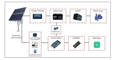
Figure 1: Block diagram of stand-alone solar PV monitoring system using IoT
