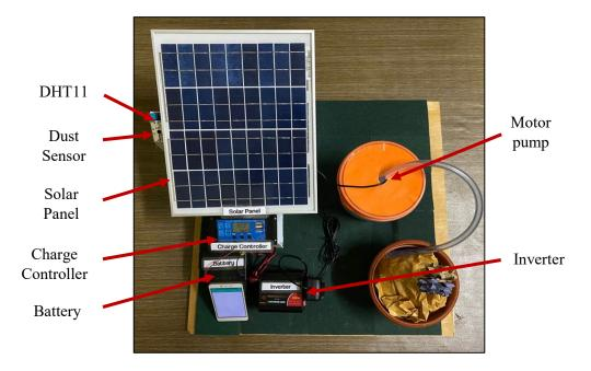
Figure 3: Prototype of solar monitoring system
