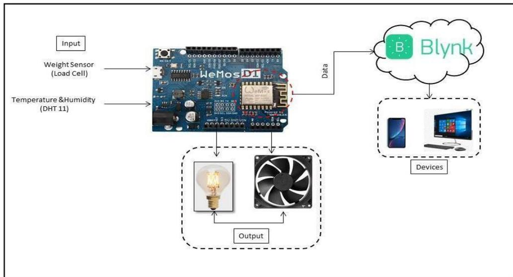
**Figure 1: Block diagram of project system design**
