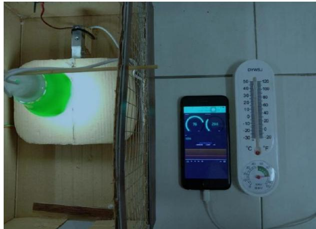
Figure 6: Measurement of temperature and humidity using thermometer and DHT11
