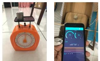
Figure 7: Weight measurement for 100g coins using weight scale (left) load cell sensor (right)
