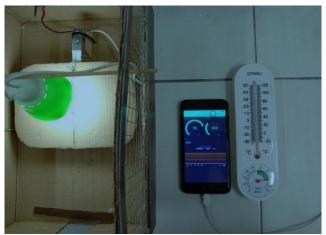
Figure 6: Measurement of temperature and humidity using thermometer and DHT11
