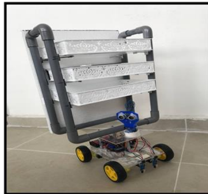
Figure 4: Food delivery monitoring system with a line follower robot
