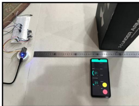
Figure 5: The measurement of the distance to detect tray and object
