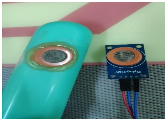
Figure 4: The old (left) and new (right) of MQ3 sensor that been used.
