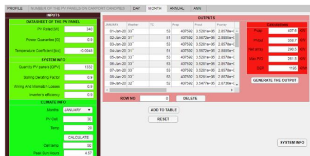
Figure 5: Prediction of carport PV power generation for one month
