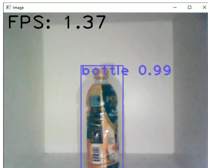
Figure 5: PET Bottle are successfully detected in the real time detection process
