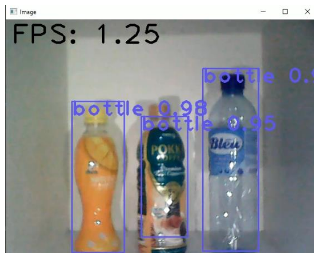
Figure 4: PET Bottle are successfully detected in the video detection process
