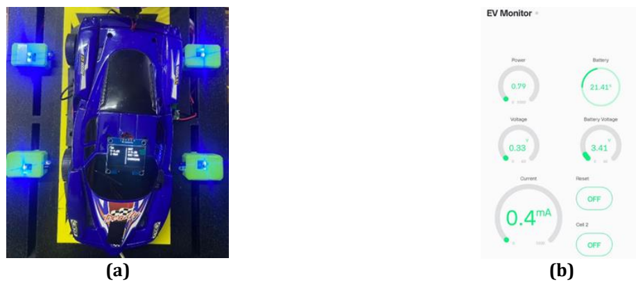
Fig. 8 System demonstration: (a) EV model correctly stationed within the parking bay and (b) live charging data presented on the mobile monitoring application
