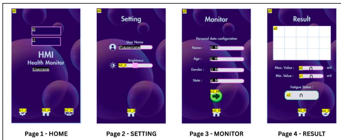
Fig. 9 GUI Implementation Using Nextion Editor
