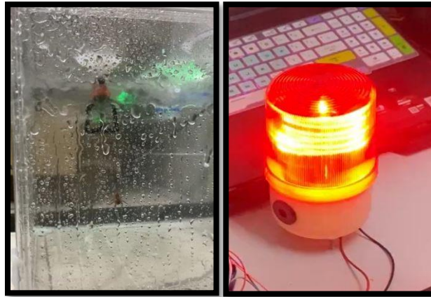
Fig. 13 Sprinkler and siren activation
