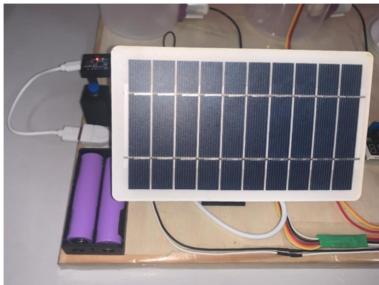
Fig. 3 The 5 V, 5 W solar panel used as the primary energy source for the solar-powered irrigation system.
