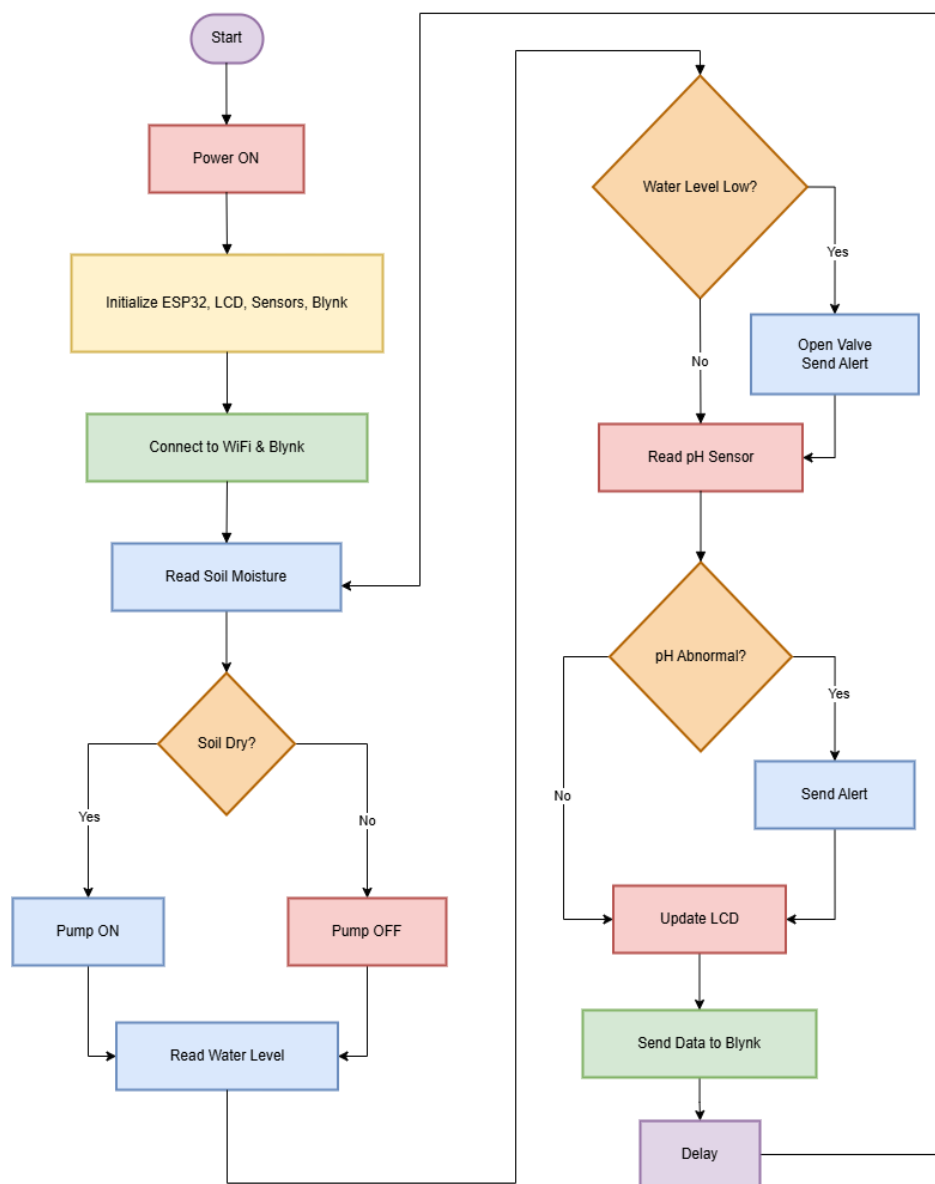
Fig. 1 Flowchart of the irrigation system working mechanism.
