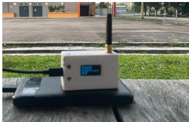
Fig. 12 RSSI testing setup in open space
