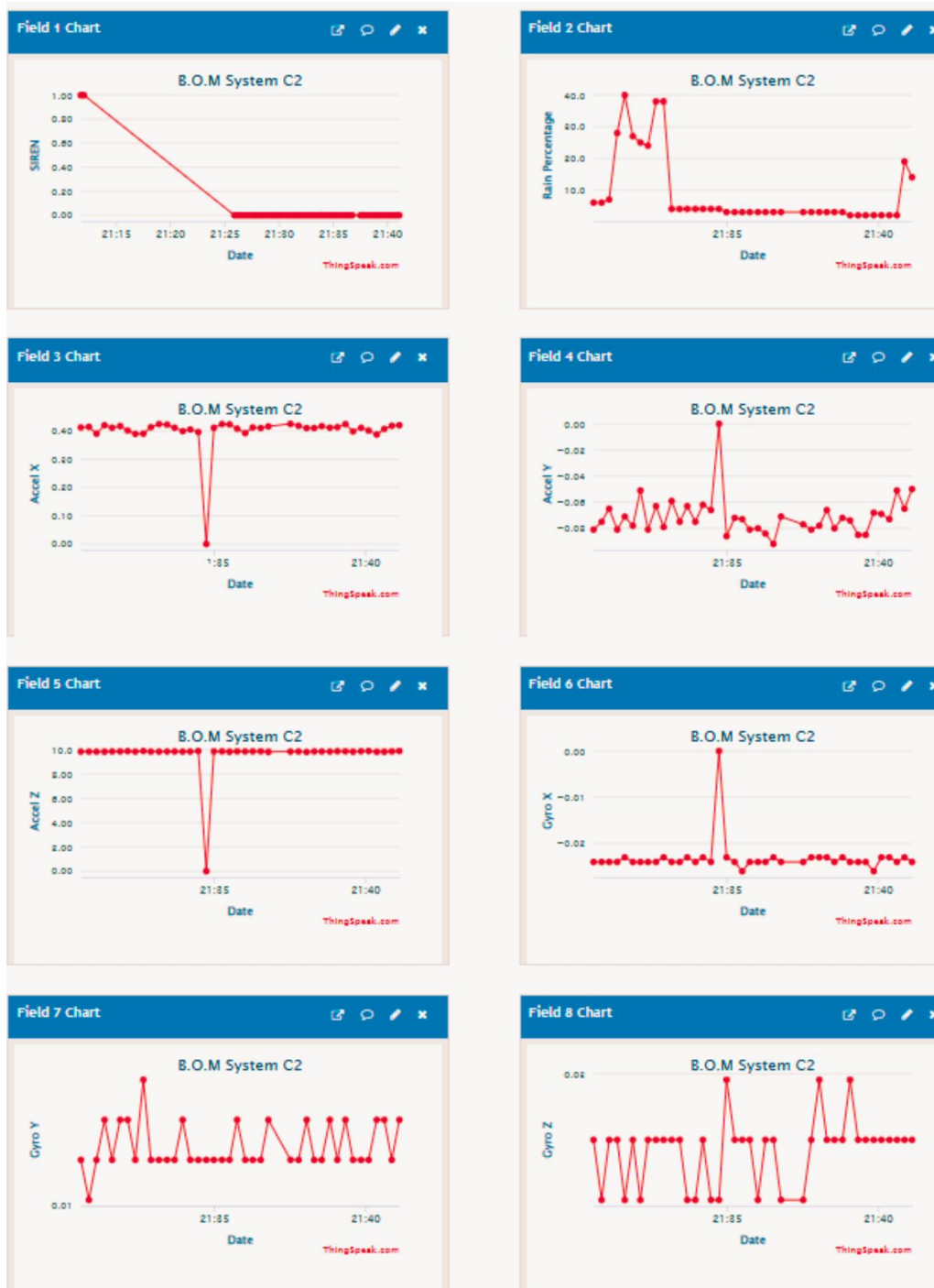
Fig. 10 Successful transmission and display of all sensor data on the ThingSpeak dashboard.
