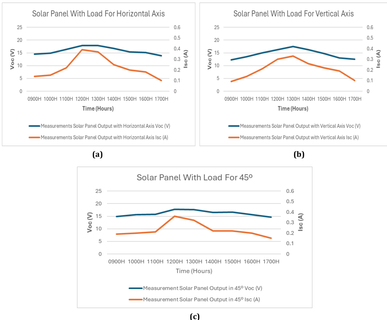
Fig. 7 Comparison Voc and Isc with load(a) Horizontal axis (b) vertical axis (c) 45 degrees
