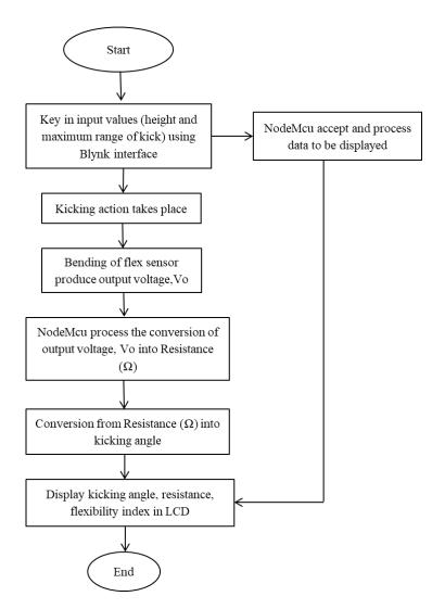
Figure 4 : Flowchart for arduino and blynk process
