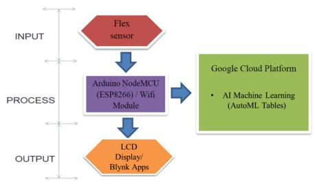
Figure 1 : Proposed functional block diagram
