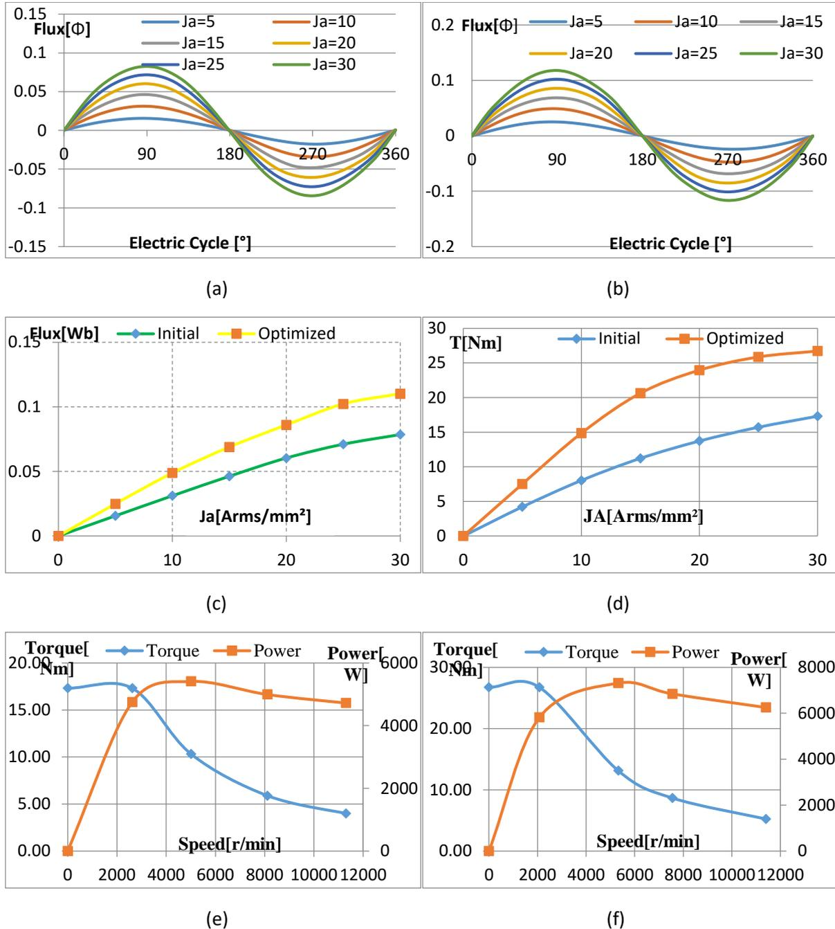
**Figure 7: Initial and optimized graph under load test (a) Initial design (b) Optimized design (c) Maximum flux at various  $J_A$  for initial and optimized design (d) Initial and optimized torque at various  $J_A$  (e) Initial torque and power vs speed (f) Optimized torque and power vs speed**
