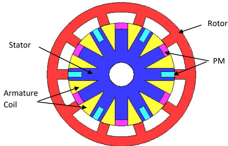
**Figure 2: Proposed 6S-10P outer-rotor AlCiRaF PMFSM (initial)**
