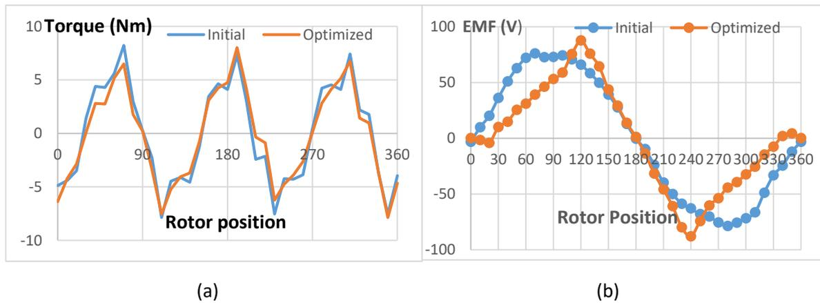
**Figure 6: No-load initial and optimized graph (a) Cogging torque (b) Induced voltage**
