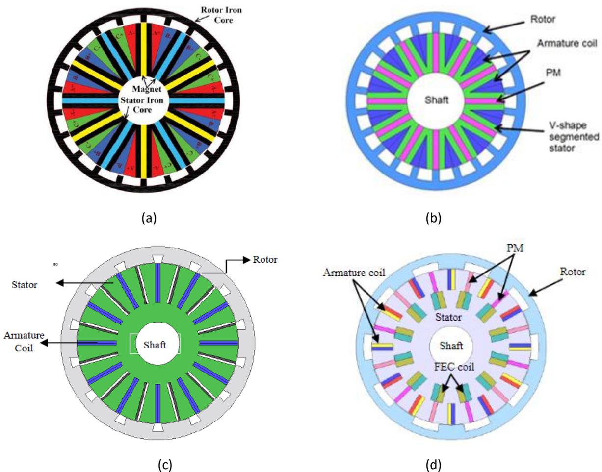
**Figure 1: Various topologies of outer-rotor flux switching machine (FSM) (a) 12S-22P PMFSM (b) 12S-24P V-shape segmented stator PMFSM (c) 12S-14P field-excitation FSM (d) 12S-14P hybrid excitation FSM**
