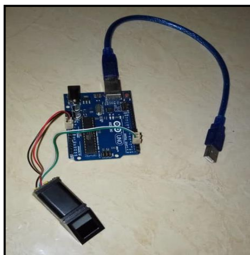
Figure 3: The connection between R307 Fingerprint Module and Arduino Uno R3
