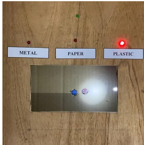
Fig.10 Paper LED is ON when the paper receptacle is full
