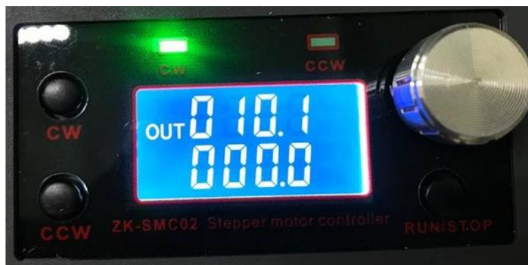
Fig. 7 Display of stepper motor controller in clockwise
