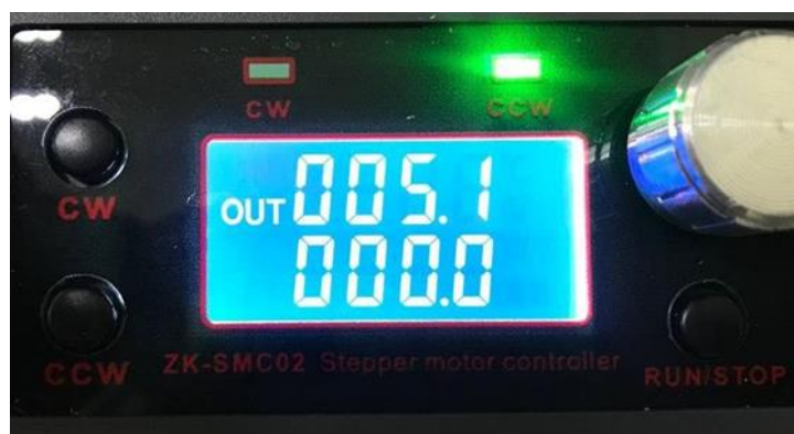
Fig. 8 Display of stepper motor controller in anticlockwise
