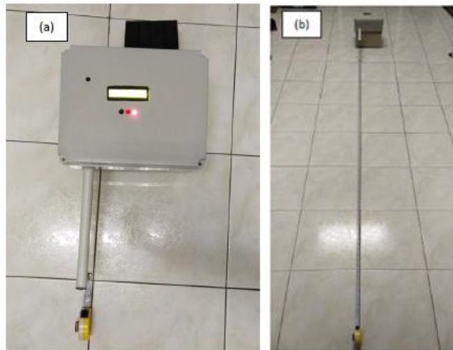
Fig. 5 Prototype indoor testing (a) Prototype placed on floor with measuring tape (b) Measuring tape's range 2M placed on floor to measure each level
