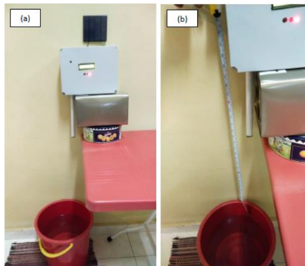
Fig. 6 Prototype indoor testing with water in pail (a) Setup for measuring 3 different water level (b) Check measured value in measuring tape and LCD
