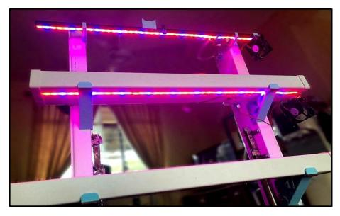
Figure 7: The grow light and ultrasonic sensor placement in prototype
