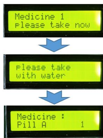
Figure 4: Display when alarm turn on
