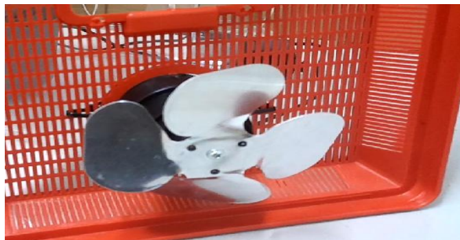
Fig. 9 Fan used as cooling component
