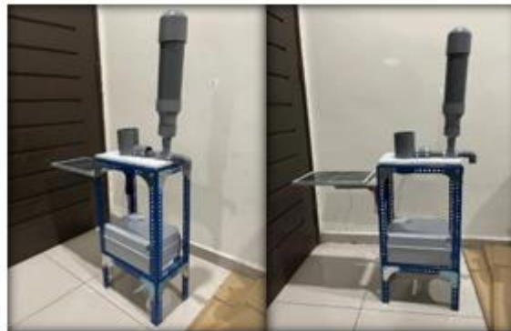
Figure 6: Full View of the automatic fish feeder integrated with Solar Photovoltaic
