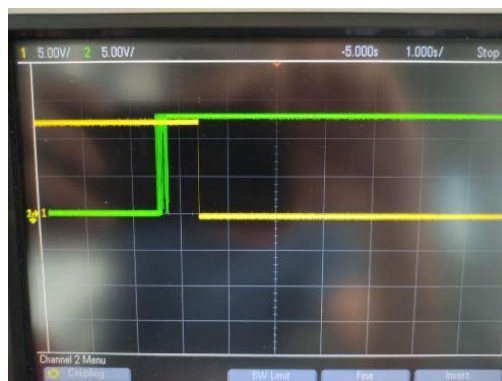
Figure 8: Waveform of load voltage upon relay 2 response
