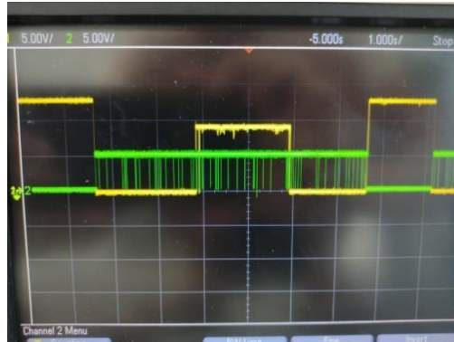
Figure 7: Response of alert signal upon battery voltage level
