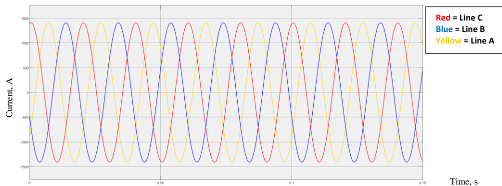
Figure 4(a): The 3-phase current waveform with no fault added to the simulation
