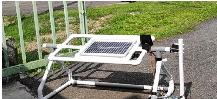
Figure 5: The PV Panel Moved According to the Sunlight.
