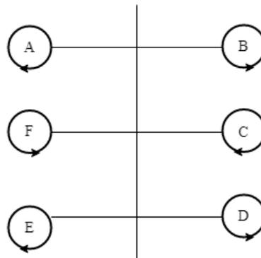
**Figure 2: The direction of rotation of the propellers for both top and bottom motors**
