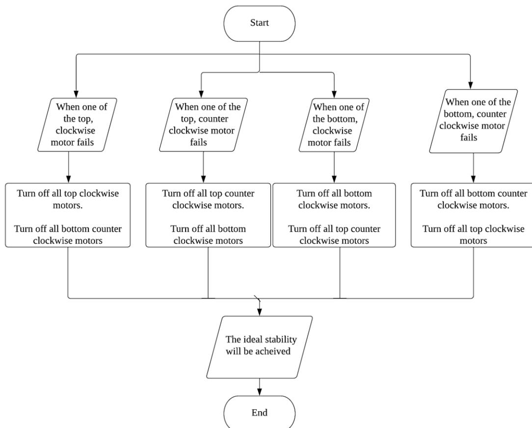
**Figure 3: Contingency counter during motor failure flowchart**
