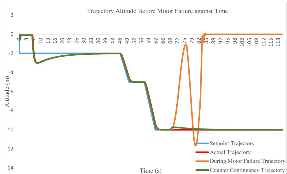
**Figure 4: Altitude trajectory for setpoint, actual, during motor failure and after counter contingency were implemented**
