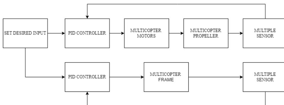
**Figure 1: The operational block diagram of the Coaxial Hexacopter H-Frame**
