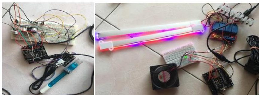
Figure 2: Hardware testing on breadboard
