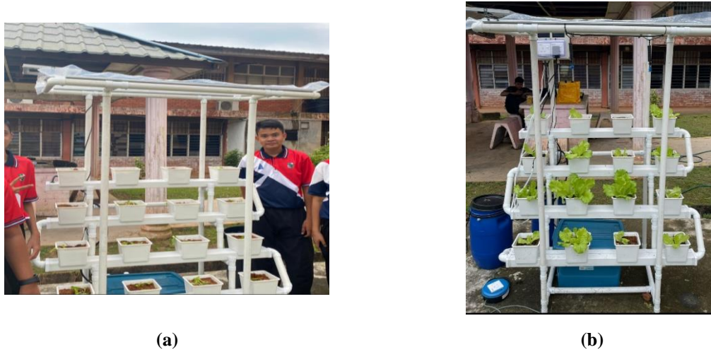
Figure 13: (a) Basic hydroponic set and (b) the installed hydroponic set with a pest control system.
