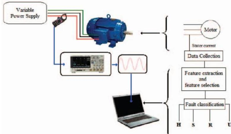
**Figure 1: Process of Current Monitoring using MCSA Method [5]**
