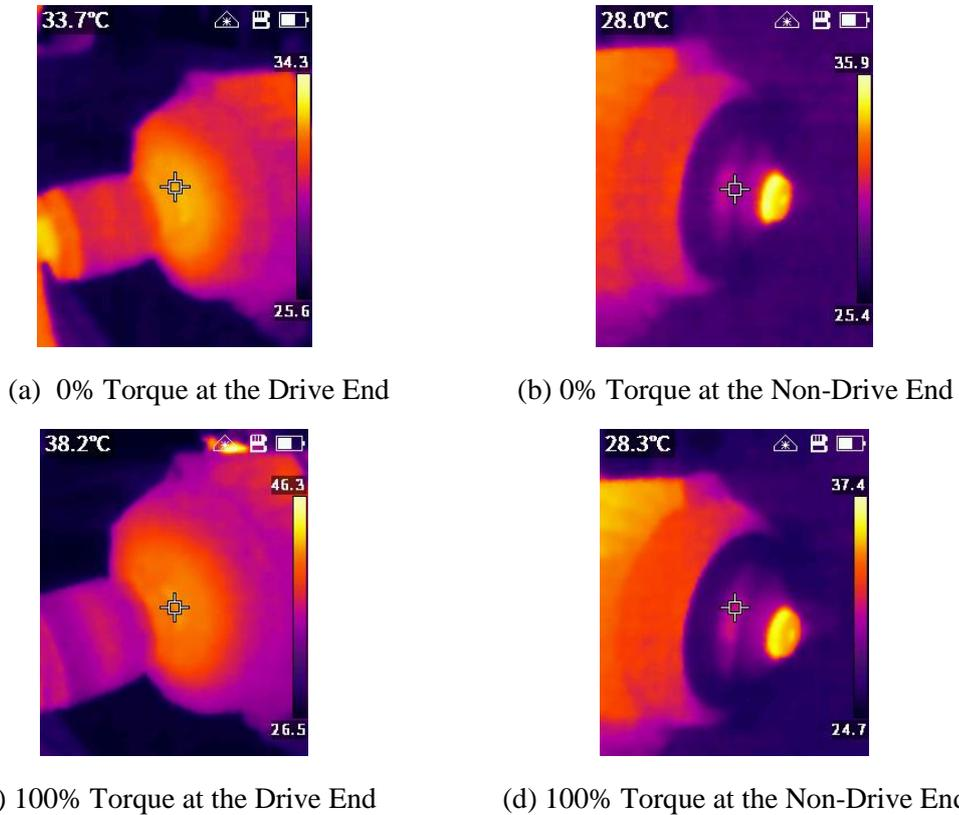
**Figure 3: Thermal Imaging for Normal condition at Drive and Non-Drive End for 0% and 100% Torque**
