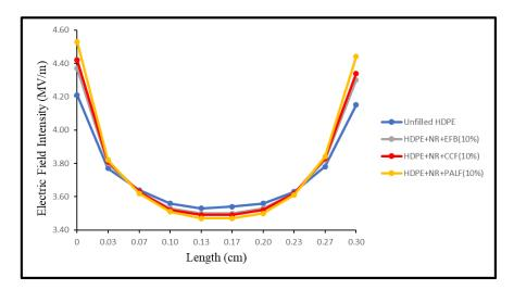
Figure 7: Comparison of electric field intensity for sample HDPE with 10% loading of biocomposites
