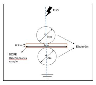
Figure 2: Geometry of electrode configuration
