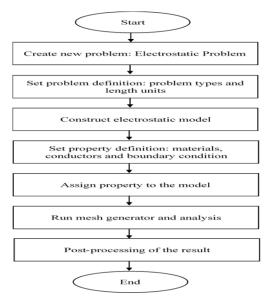
Figure 3: Steps for designing 2D axisymmetric problems in electrostatics
