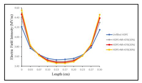
Figure 4: Electric field intensity for HDPE with 10%, 20%, and 30% of oil palm empty fruit bunch with unfilled HDPE as a reference
