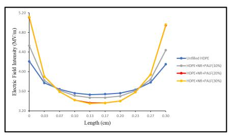
Figure 6: Electric field intensity for HDPE with 10%, 20%, and 30% of pineapple leaves fibre with unfilled HDPE as a reference
