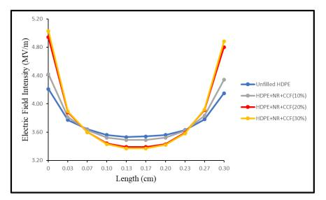
Figure 5: Electric field intensity for HDPE with 10%, 20%, and 30% of coconut coir fibre with unfilled HDPE as a reference
