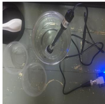
Figure 11: EC sensor test on nutrients
