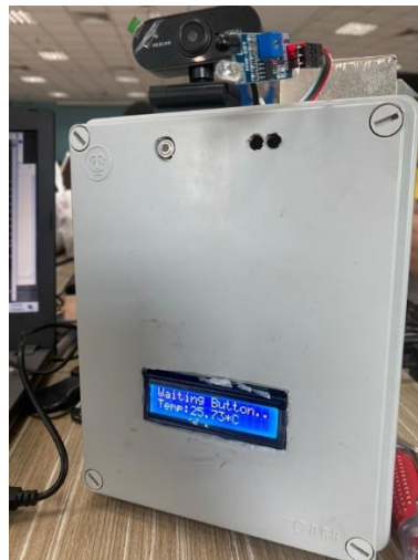
Figure 3: Prototype design for facemask and temperature detector
