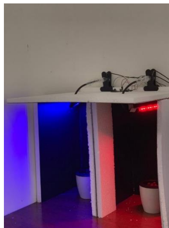
Figure 1: The prototype of the LED grow lights automation
