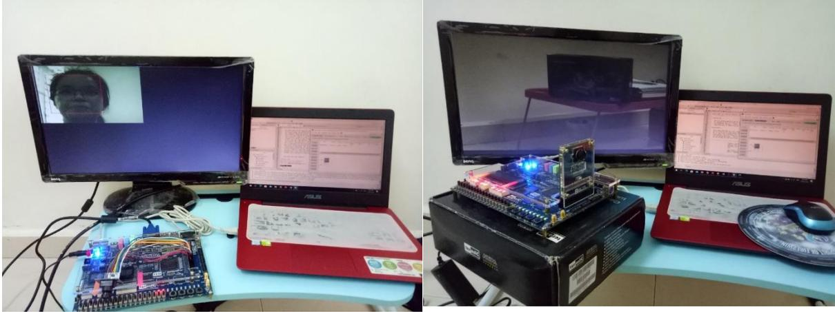
**Figure 2: Overall connection of DE2-115 board with (a) OV7670 (b)TRDB-D5M**
