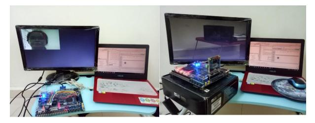
Figure 2: Overall connection of DE2-115 board with (a) OV7670 (b)TRDB-D5M
