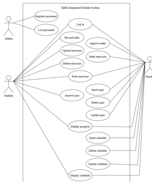
Fig 2 Use-case Diagram for Tahfiz Integrated Module System
